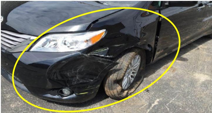
Figure 3 - Damage to the subject Toyota Sienna (area of damage circled)
